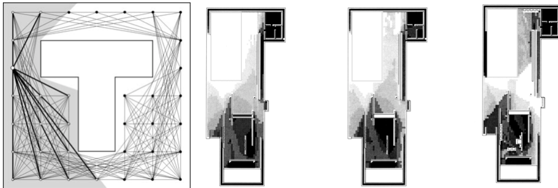
Figure 22: Example results from the work of Turner et al. [148] on isovists and visibility graphs. Left: An example of a first-order visibility graph, showing the pattern of connections for a simple configuration. Right: Mies van der Rohe's Barcelona Pavilion showing neighbourhood size (left), visibility mean shortest path length analysis (middle), and accessibility mean shortest path length analysis (right). Source: [148]
