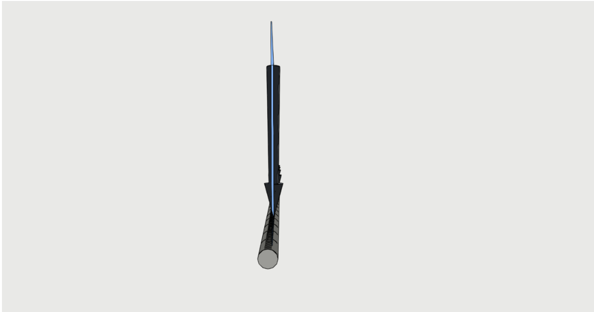
Figure 3.6.3g - 3-Dimensional Line Loads. 3-D arrows attempt to solve the issue of looking at the element from the side.
