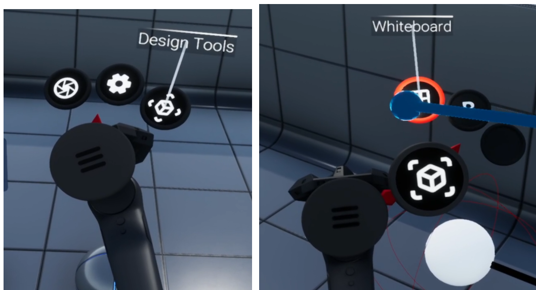
Figure 12: The radial menu allows to place theoretical infinite functionalities as it is developed to show functionalities in a cascaded form.
