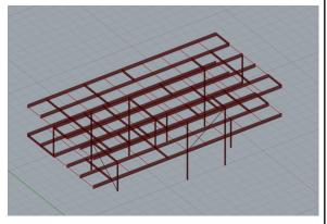
An example of an infeasible solution, which utilises a few bracings and secondary beams.
