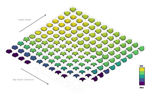
As expected the fittest solution is high and symmetric, however, in this case the arches are low to form a dome, and the fittest region has moved back to being high, but only so high that it can have flat side arches.. The colour map again shows the relative fitness. To see how the solutions evolved over time, the image below shows the map after 1000, 5000, 10,000 and 100,000 iterations.
