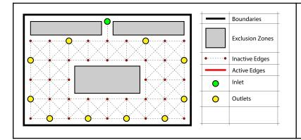
Problem specification of an MVS, including the outer boundary, the exclusion zones, a set of potential connections and the positions of the inlet and outlets.
