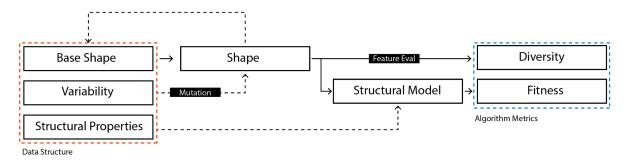
The data structure stores the information on the left to enable shape manipulation and automated generation of a structural model for simulation. The shape provides the basis for feature evaluation and the structural properties include loads, materials and support conditions. At each mutation a new object with an updated base shape is generated.
