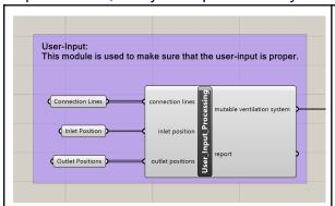
The "user-input-processing" component that pre-processes the user's input-sketch.
