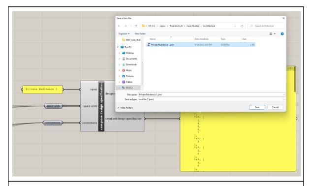
Screenshots showcasing how a Design Specification can be saved to disk, using the custom menu element of the "compose design specification" rhino component. Furthermore, as shown in the screenshot at the top, a preview of the output json file can also be inspected from within the grasshopper environment.
