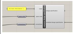
Close-up view of the "compose design specification" component, showcasing its three input variables: a name, a list of space units and a list of connections.
