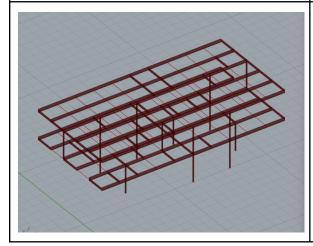
An example of a feasible solution, which utilises a few bracings and secondary beams.
