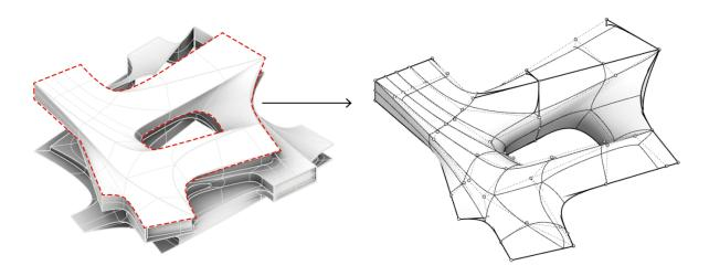
To work in a reasonable way within the QD process the geometry was simplified in order to reduce the complexity of the problem. Some additional control points were added to ensure the desired variability is included from a structural point of view, and in addition some redundant control points were removed. The final model with added point constraints and variations is shown in the images below. On the left the control mesh is shown and on the right the high resolution (smooth) geometry.
