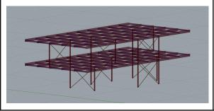
Isometric view of the initial karamba stick-model that is used as input to the QD algorithm.
