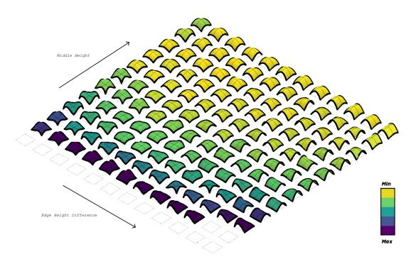
The figure above shows the map of feasible solutions, with a colour map showing the fitness (elastic energy) with yellow being the "fitter" solutions as these show a higher stiffness (low elastic energy). The map shows the importance of height and the best performing solutions are as expected found in the top left corner where the features correspond to the solution being high and symmetric. However, it can be seen that asymmetric vaulted solutions can be used with little trade off in stiffness.
