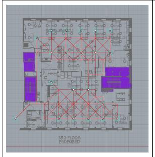
An example definition of a Mutable Ventilation System in Rhino's design environment.
