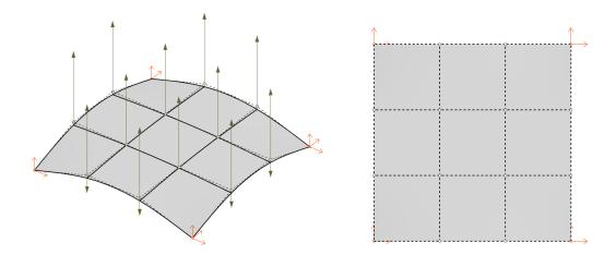
The structure is analysed as a structural shell with pinned supports located at each corner. The structural analysis process is set up with the following properties:
