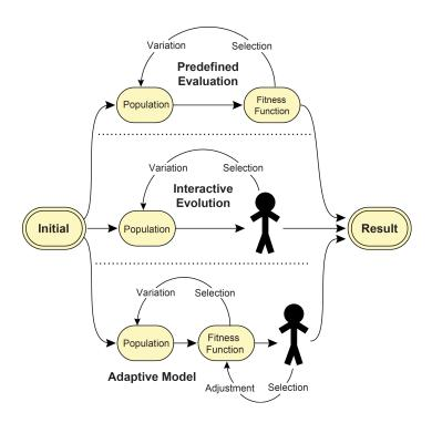
Functional diagram showcasing three approaches to search-based procedural content generation: 1) Predefined Evaluation, 2) Interactive Evolution, where the user replaces the evaluation method and (3) *Adaptive Model* where the user's input adjusts the fitness function which, in turn, ranks content by a personalized measure of quality. Source: [1]
