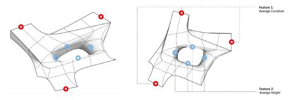
To capture the features of the villa model, the focus was therefore put on two areas which could have significant impact on both the architectural design aspects and the structural performance, which are the curvature of the framed window portions and the height of the middle "funnel".
